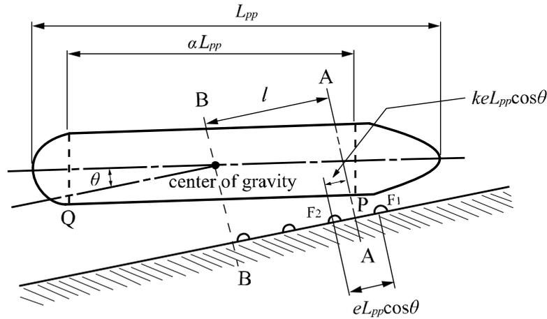
Fig. 2.2.5 Schematic Illustration of Ship Berthing<sup>10)</sup>
