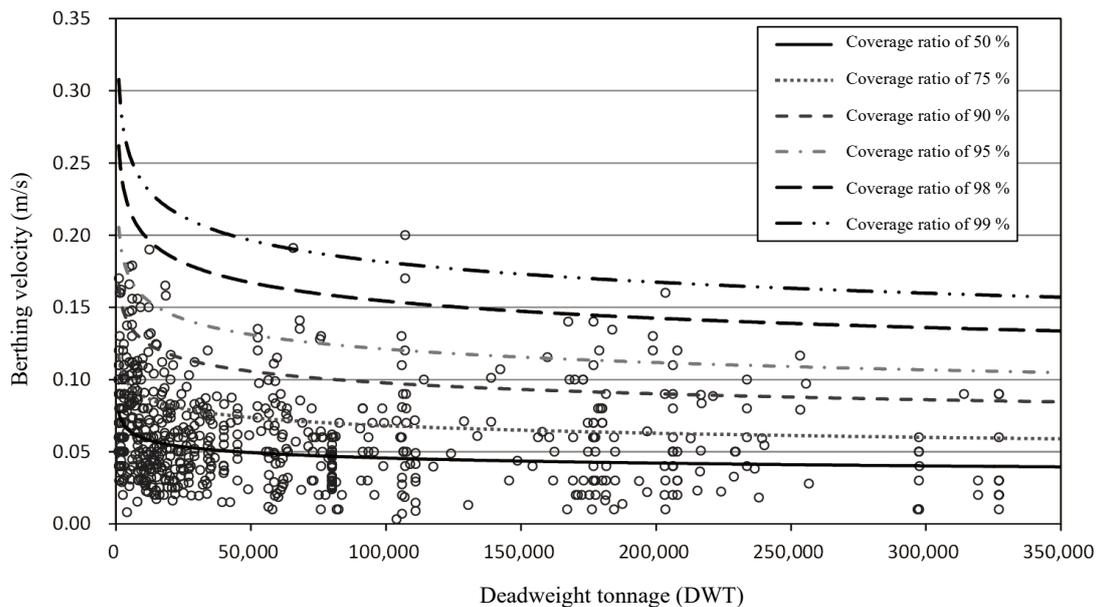
Fig. 2.2.3 Relationship between Measurement Values of Berthing Velocities of Ships and Regression Equations<sup>6)</sup>
