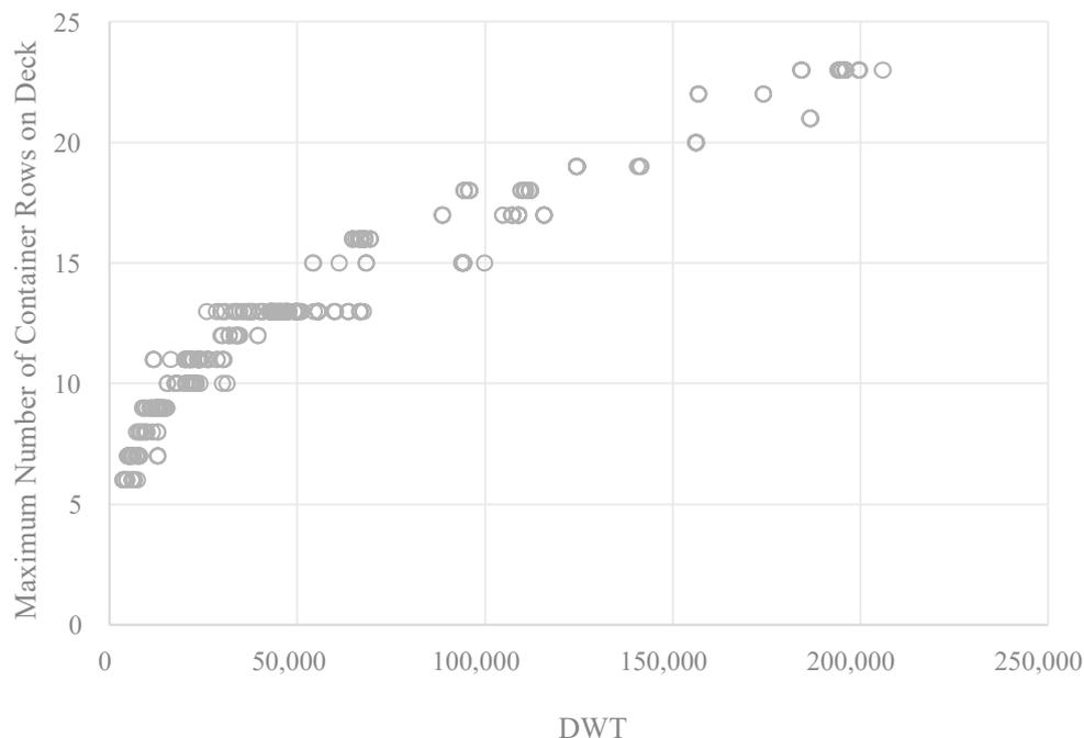
**Fig. 1.2.2** Correlation between Deadweight Tonnages and Maximum Number of Container Rows on Deck in Container Ships
