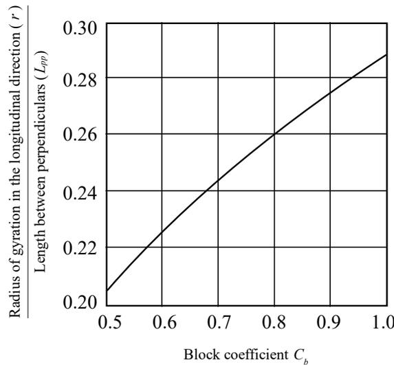
**Fig. 2.2.4** Relationship between Radii of Gyration in the Longitudinal Direction and Block Coefficients<sup>9)</sup>
