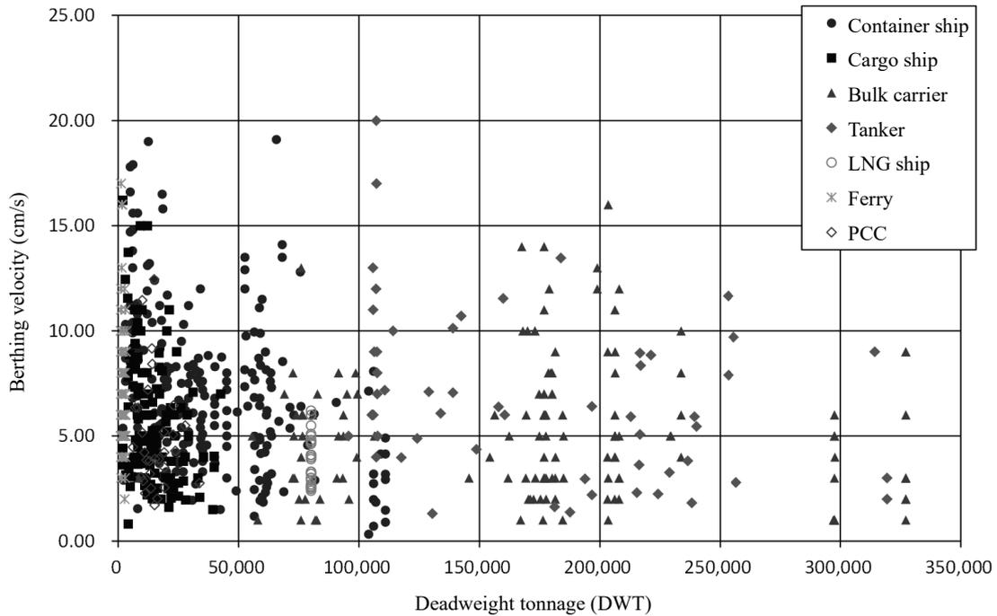
Fig. 2.2.2 Measurement Values of Berthing Velocities (by Ship Type)<sup>6)</sup>
