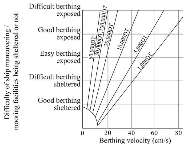
**Fig. 2.2.1** Relationship among Ship Maneuvering Conditions, Ship Sizes, and Berthing Velocities<sup>3)</sup>
