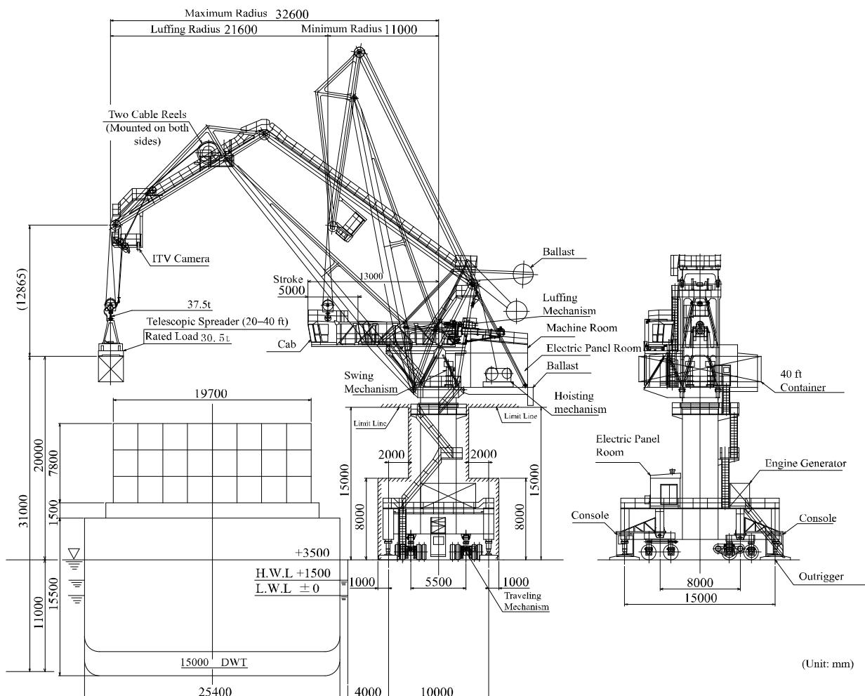
Fig. 3.2.9 Example of a Tire-Mounted Multipurpose Jib Crane
