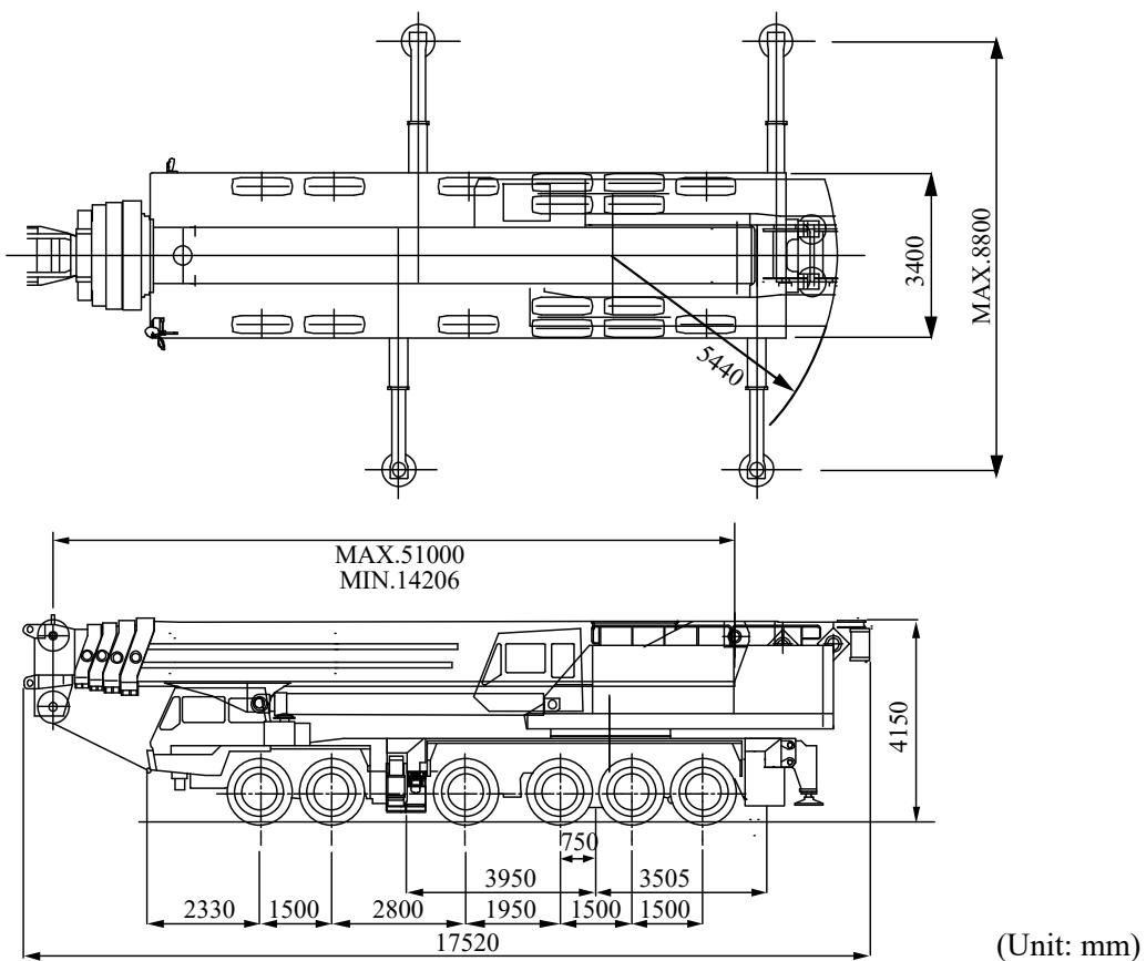
**Fig. 3.2.12 Example of a Truck Crane****Table 3.2.7 Examples of the Dimensions of Rough-Terrain Cranes, All-Terrain Cranes, and Truck Cranes**
