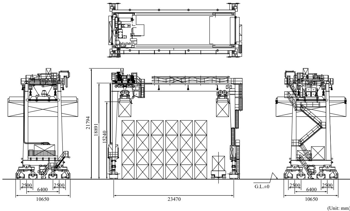
**Fig. 3.2.15** Example of a Transfer Crane**Table 3.2.10** Examples of Dimensions of Transfer Cranes
